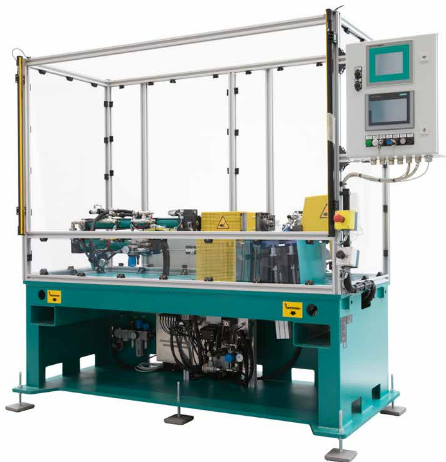
Press-in machine for turbocharger housings
