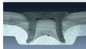
Cross-section of a semi-hollow punch rivet connection.
